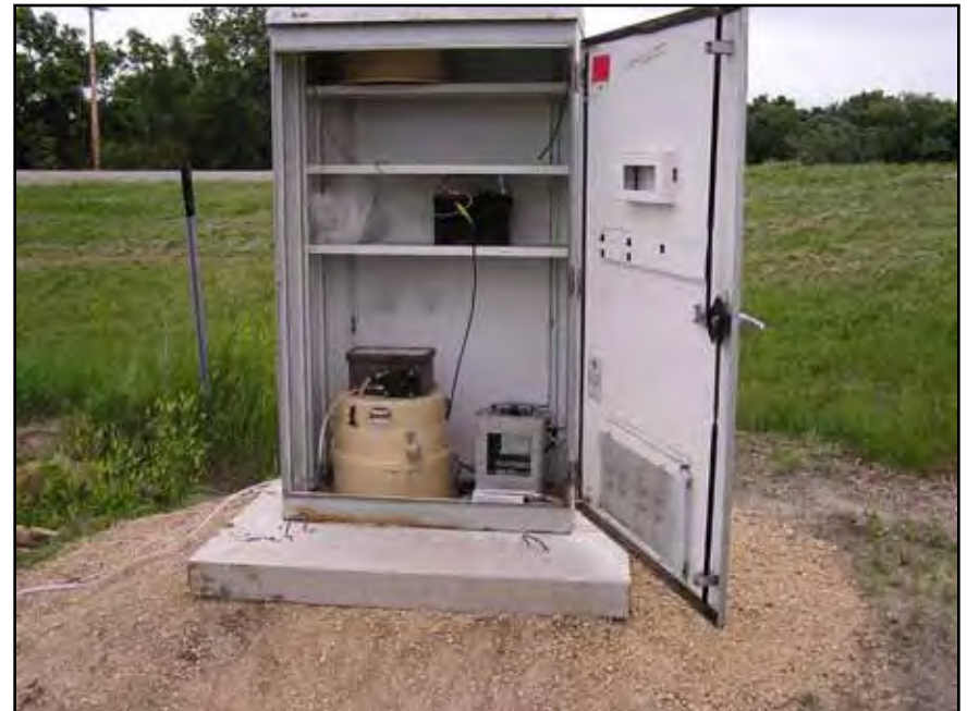
Monitoring cabinet permanently installed near a rain garden.
