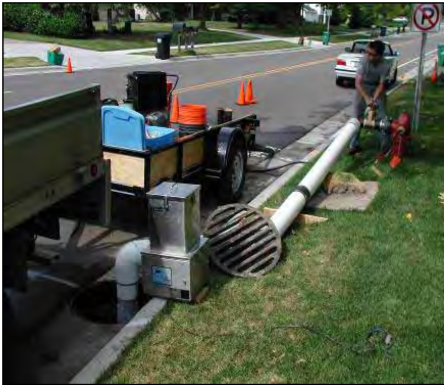
Synthetic runoff testing using a fire hydrant and controlled sediment feeding
