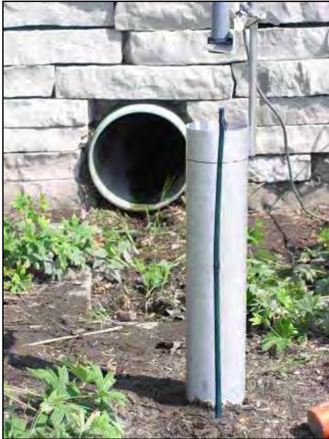
Modified Philip-Dunne Infiltrometer measuring hydraulic conductivity
