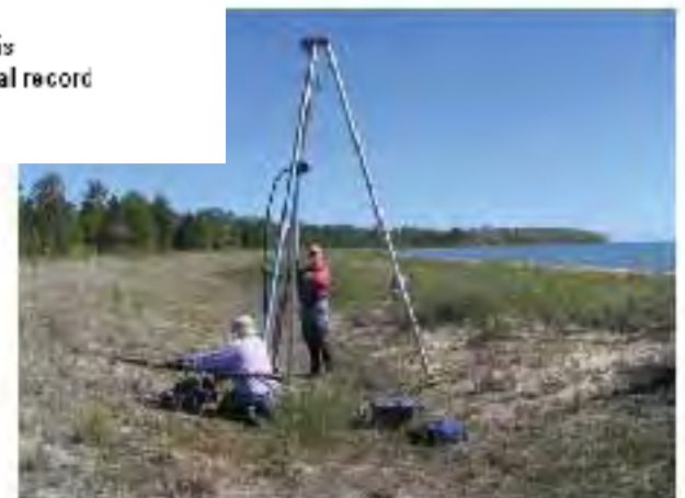
Vibrocoring at Nequigon State park, Michigan. Vibrocoring is an important tool needed to understand the subsurface geology of coastal systems throughout the Great Lakes.
