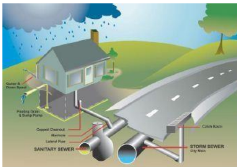
Sanitary and Storm Sewer Systems
